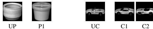
Figure 3. The two unknown objects "car3" (UC) and "uncovered pot" (UP) omitted from the training set together with their visually most similar objects (according to the distance within the Eigenspace) "car1" (C1), "car2" (C2) and "half covered pot" (P1) contained in the training set.
