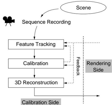
Figure 1: Calibration steps with main data path and possible feedback loops.
