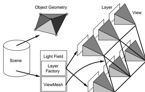
Figure 2: Common components of a scene model. Starting from the scene database, the arrows represent the object interconnections.
