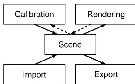
Figure 3: Modules of lgf3. The solid lines denote the main data paths. The dashed lines mark the feedback loop.
