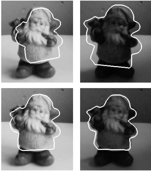
Figure 7: The upper images show results of tracking without basis images and the lower images show results using basis images. The benefits of the basis image approach is clearly visible.
