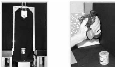
Fig. 1. Left: turntable with camera arm. Right: hand-held camera.
