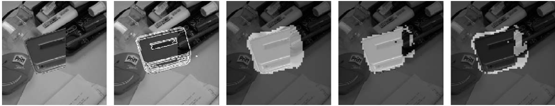
Fig. 14. From left: hole punch partially occluded in heterogeneous background; pose estimated by the object recognition system; respective trained bounding region O ; these feature vectors marked gray (inside the bounding region) are assigned to the object; the others are assigned to the background.
