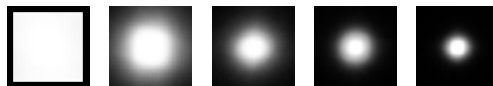
Figure 5: Basin of convergence of motion estimation algorithms for maximum feature displacement of ten pixels, brighter intensities denote higher percentage of successful tracking. Algorithms from left to right: bm coef , gd trans , gd trans + ill , gd affine , gd affine + ill .
