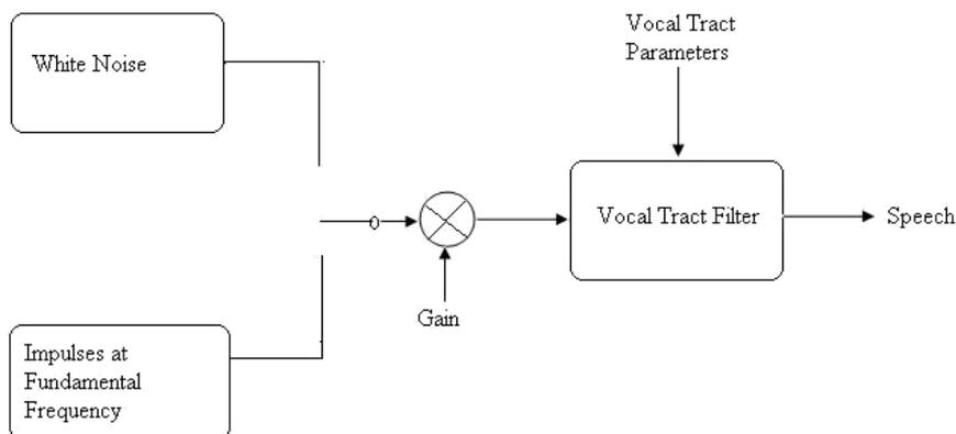
Figure 1: Diagram of the source-filter model (after [4])
