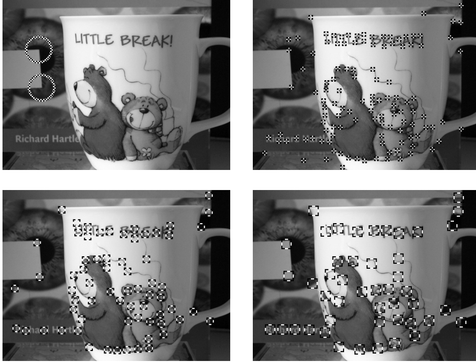
Figure 3.5: The results of feature selection for the interest images of Figure 3.4. All features windows have a minimum distance of 12 pixels from each other. The two highlighted areas illustrate the phenomenon that corners inside a feature window are often positioned at its very edge, which is especially prominent for the large feature windows in the lower right image.
