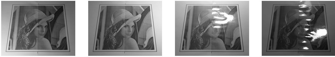
Figure 2.9: The four images of this figure show a planar test target, which has a non-specular surface on the left side and a highly specular surface on the right side. The appearance of the specular surface changes vigorously when it reflects the light rays from the light source to the camera.
