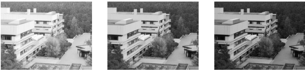
Figure 6.2: In addition to the images captured with standard exposure settings (middle image), every static test scene was slightly overexposed (left image) and underexposed (right image). The resulting images are used to evaluate the robustness of the individual motion estimation algorithms to intensity changes in the feature windows.
