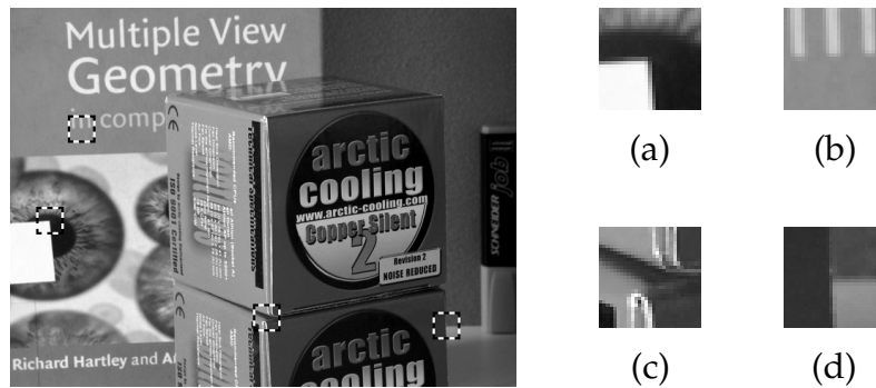
Figure 3.2: This figure illustrates potential problems in relating a 2-D feature window to a unique 3-D feature point. The feature windows (a) and (b) both lie on a planar surface. Feature window (a) also has a unique texture, which is the ideal case for feature point tracking. However, feature window (b) looks exactly like an image region to its right, which can lead to erroneous feature correspondences. Although the feature windows (c) and (d) do not lie on a planar surface, feature window (c) can be reliably attributed to a unique 3-D feature point. In contrast to this, feature window (d) spans across a depth discontinuity and does not represent a unique point in 3-D space.
