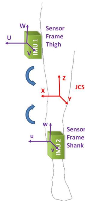
**Figure 2: Two inertial measurement units are placed on the thigh and shank, which form their own local coordinate system. To compute the joint angle, the sensor frames are transformed in a mutual coordinate system, the joint coordinate system (JCS).**
