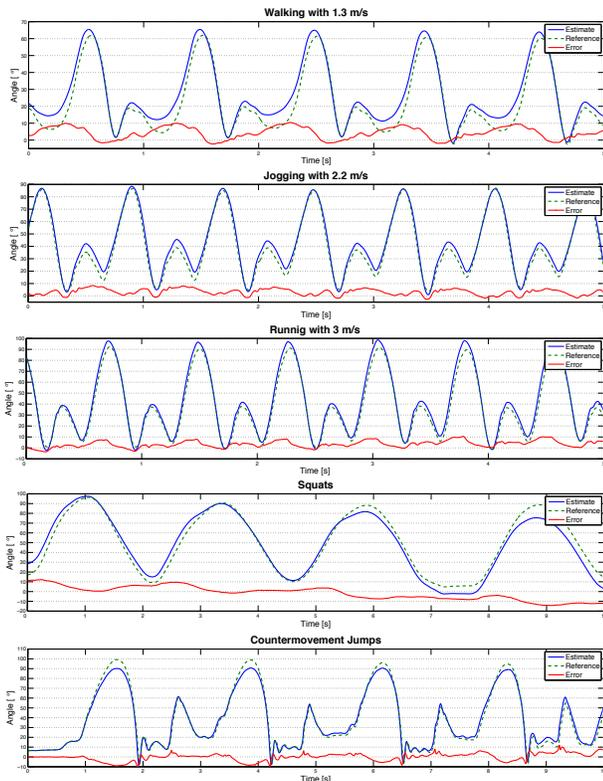
**Figure 5: Knee angles computed by the algorithm compared to the camera reference knee angles from the camera system for one subject performing all five dynamic movements. Additionally the knee angle estimation error is shown.**
