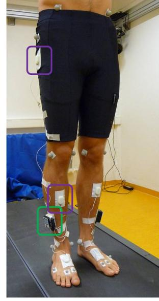
**Figure 3: Attachment of the IMUs (top and middle box) and the data logger (bottom box) during data collection. The IMU of the shank was positioned four centimeters under the trochanter major, while the IMU of the thigh was positioned four centimeters under the middle of the frontal tibia. For the reference system, 32 reflective markers were attached to the leg.**
