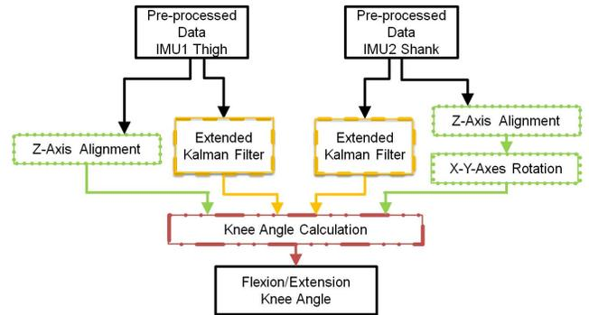
**Figure 1: An overview of the calculation of the knee angle from the two IMUs at the thigh and shank. The procedure can be divided into three main steps: the alignment procedure, the extended Kalman filter, and the knee angle calculation.**
