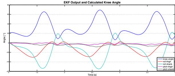
Figure 4: Flexion/extension knee angle calculated using the outputs of the EKF roll and pitch of thigh and shank during walking at 1.3 m/s.
