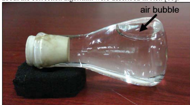
Fig. 4. The conical phantom (bottom diameter: 300 mm, height: 600 mm) used for the reconstruction image evaluation.
