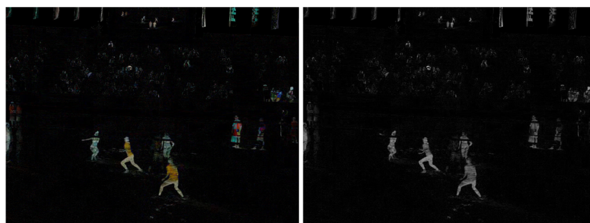
Figure 3. Difference image obtained from subtraction of the background image from the current frame (left), and then single channel grayscale converted (right).
