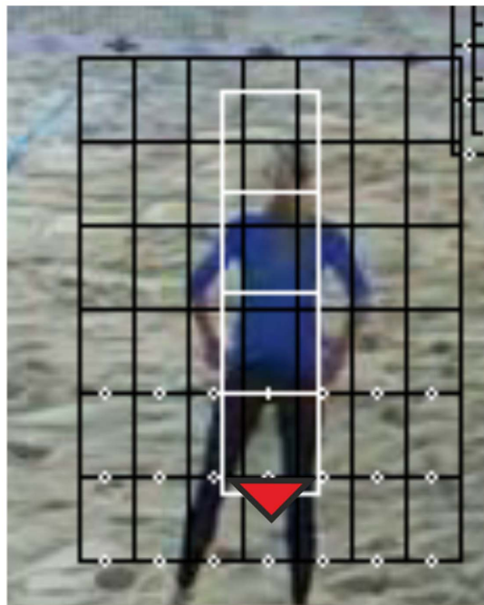
Figure 6. Screenshot of the tracking of one of the players by means of the integral histogram approach. The grid is shown on the original frame for illustration purposes, while the tracking is actually done on the foreground mask filtered frame to suppress the background from the calculations.
