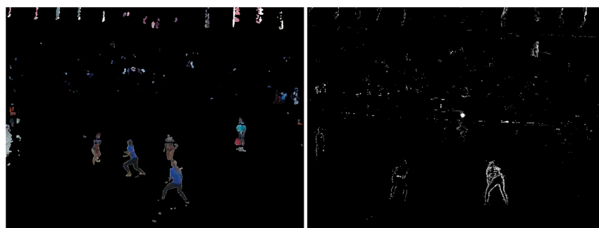
Figure 5. Final result after applying the foreground mask to the current frame of the video (left) and binary image showing pixels differing from the previous frame and used for calculating the movement weight for each particle (right).
