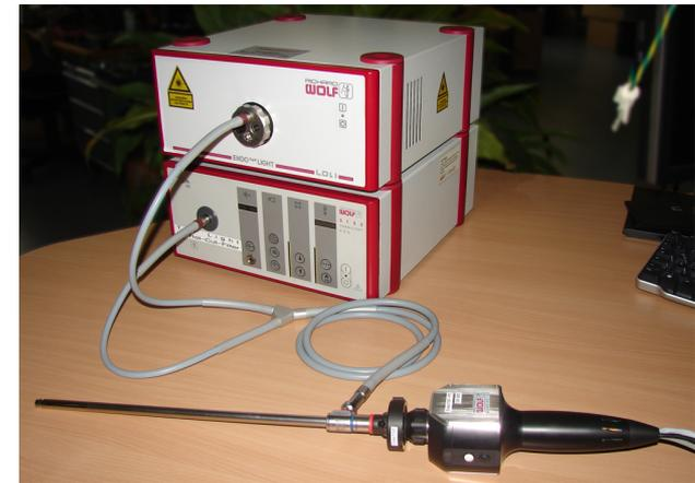
ToF/RGB endoscope prototype
