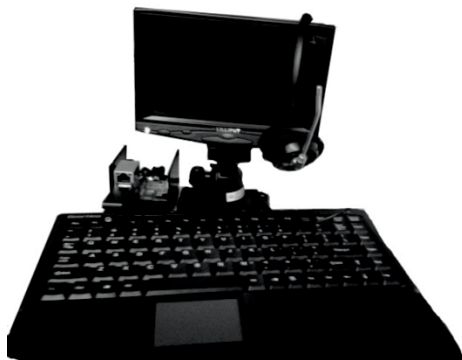
Figure 7 Portable device for the analysis of speech of people with PD
