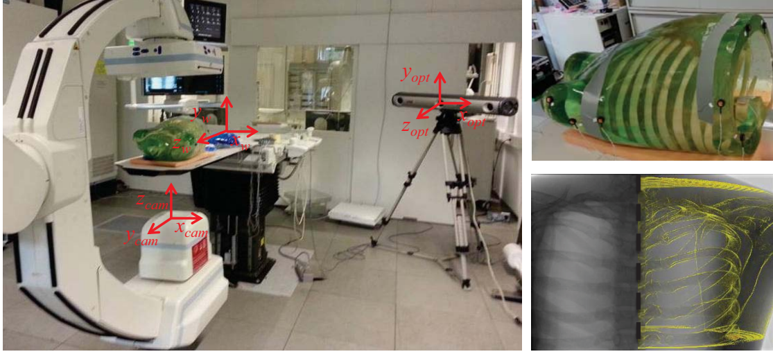
Figure 4. An interventional C-arm system is used to acquire both 2-D image sequence and 3-D C-arm CT volume of a thorax phantom. Motion of the thorax phantom is triggered manually. The OptoTrak motion capture system is used to acquire the ground truth.
