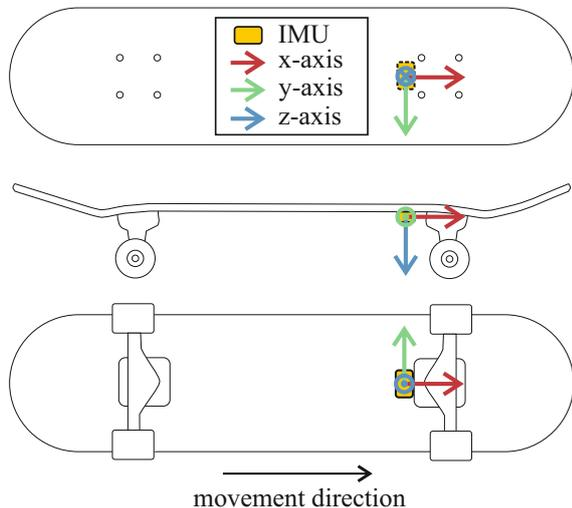
**Figure 1: Sketch of the inertial sensor attachment including visualization of the sensor axes (not drawn to scale).**
