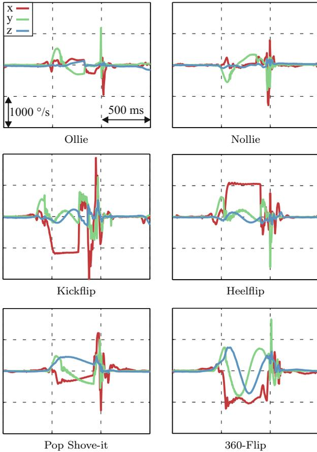
Figure 2: Example gyroscope signals of one subject of all tricks that were used for the classification analysis.
