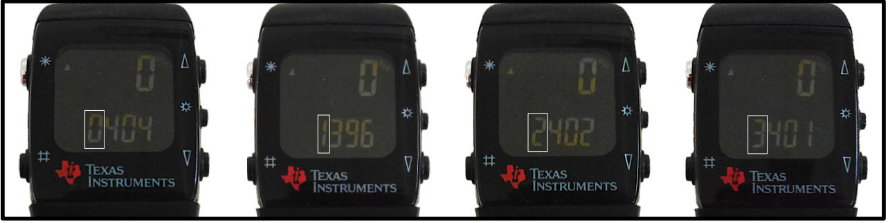
Fig. 3 CHRONACT systems displaying the classification results of 0 (LOW-STA), 1 (LOW-ACT), 2 (MED) and 3 (HIGH). Additionally, the devices show memory consumption (top right) and debug information for radio communication (bottom right).
