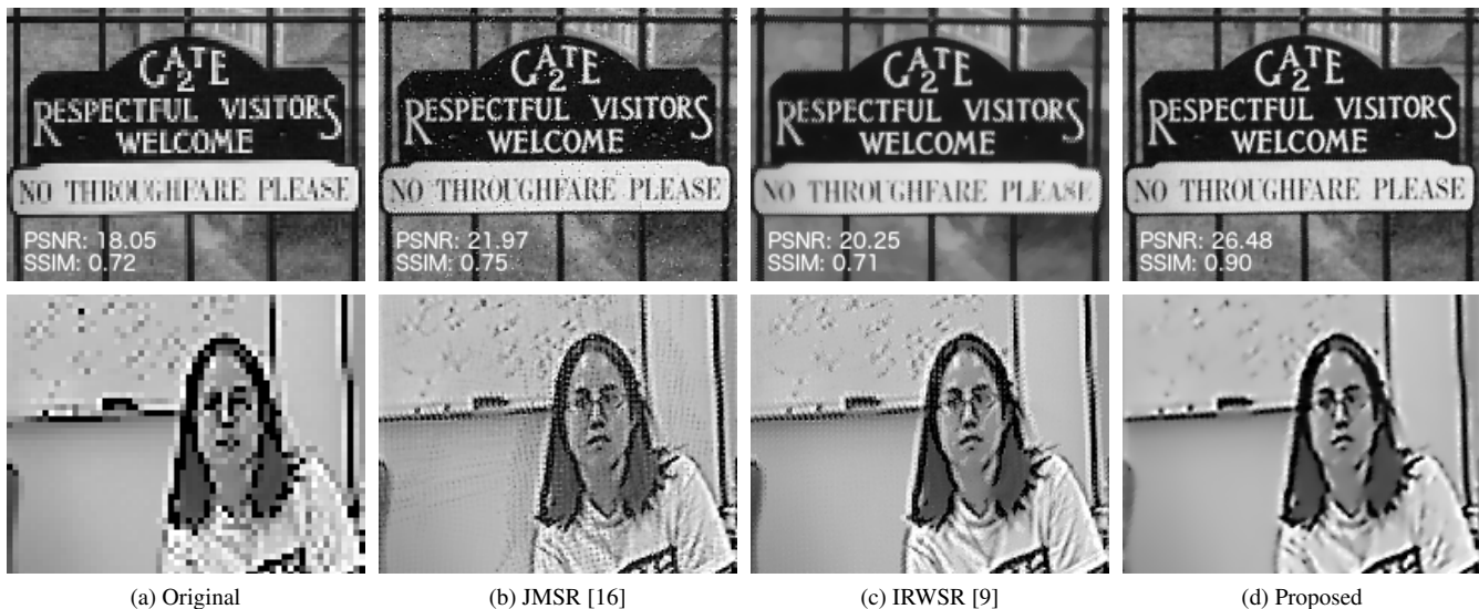
Fig. 3: SR reconstructions provided by the competing algorithms on simulated and real datasets. Top row: Simulated dataset with uncertainties in the initial motion parameters and outliers due to invalid pixels generated by salt-and-pepper noise. Bottom row: Emily dataset with outliers due to non-rigid motion across the LR frames related to movements of the head.
