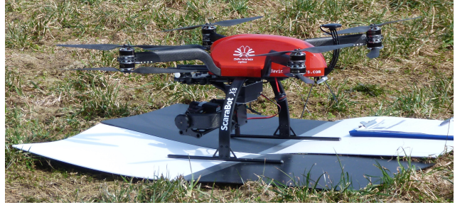
Figure 2. Remote-controlled octocopter with an integrated infrared and RGB camera, which we use for data acquisition.
