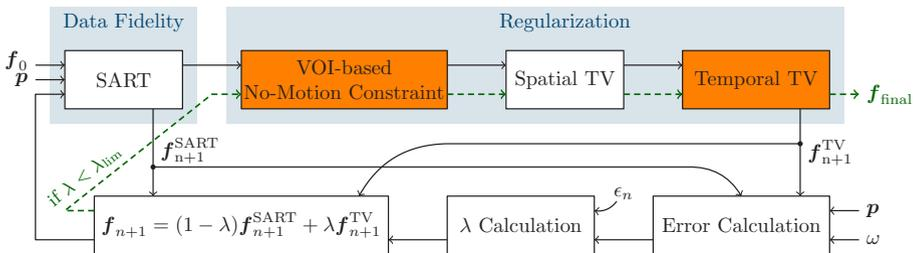
**Fig. 1.** Sequence diagram of the extended iTIV algorithm. The new temporal regularization parts are highlighted in orange. When the stopping criterion  $\lambda < \lambda_{\text{lim}}$  is reached,  $\mathbf{f}_{\text{final}}(t)$  is calculated using the dashed green path.
