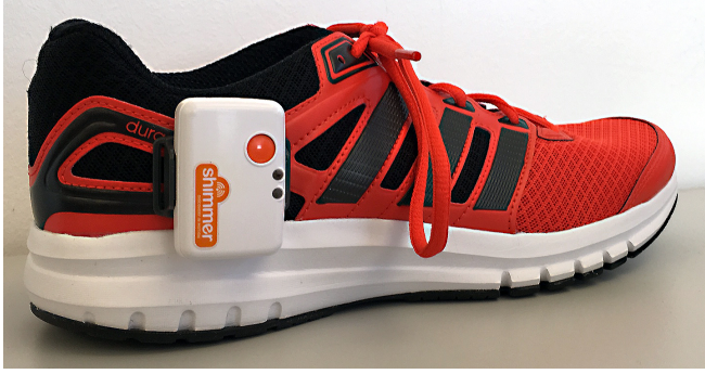
Fig. 1. A Shimmer ® 3 inertial sensor platform was mounted on the lateral side of each foot.
