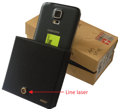
Fig. 1: The optical based laser rangefinder which is composed by two main elements: an Android device and a laser line emitter placed on the bottom of the device and aligned exactly perpendicular to the smart phone camera.
