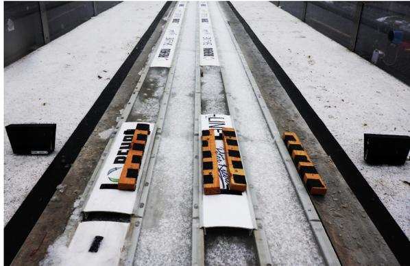
Fig. 2. Magnetic gate in combination with a light barrier system. IMMUs and global time were synchronized by evoking a distinct peak in the magnetometer signal while at the same time triggering the light barrier.
