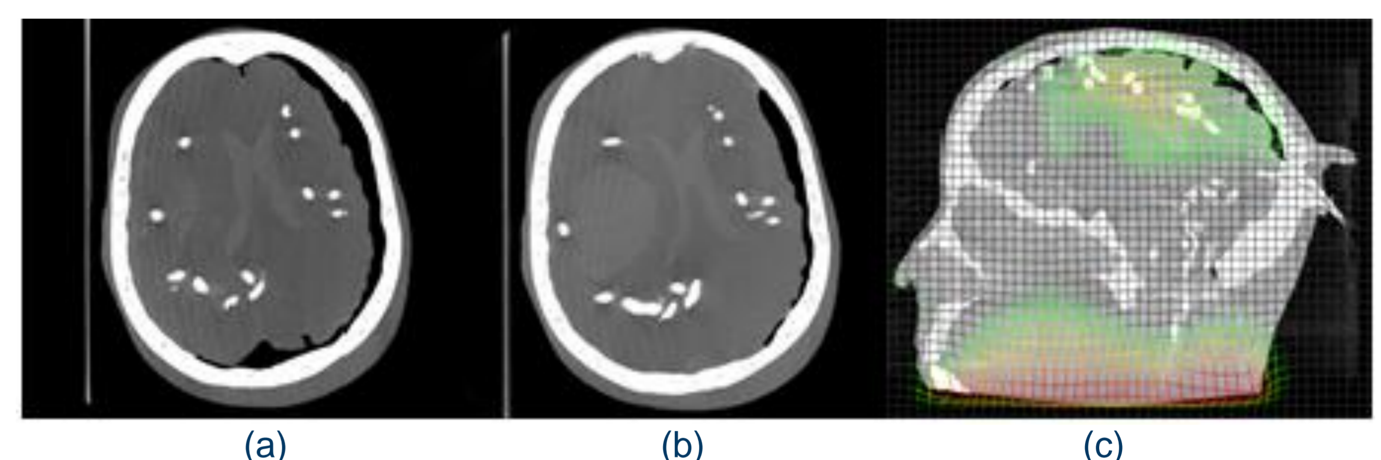
Figure 4: Examples of CBCT (a)-(b) phantom acquisitions. (a) shows the acquisition with maximum deflated tumor, while (b) presents the maximum inflated tumor, (c) shows the estimated displacement field.
