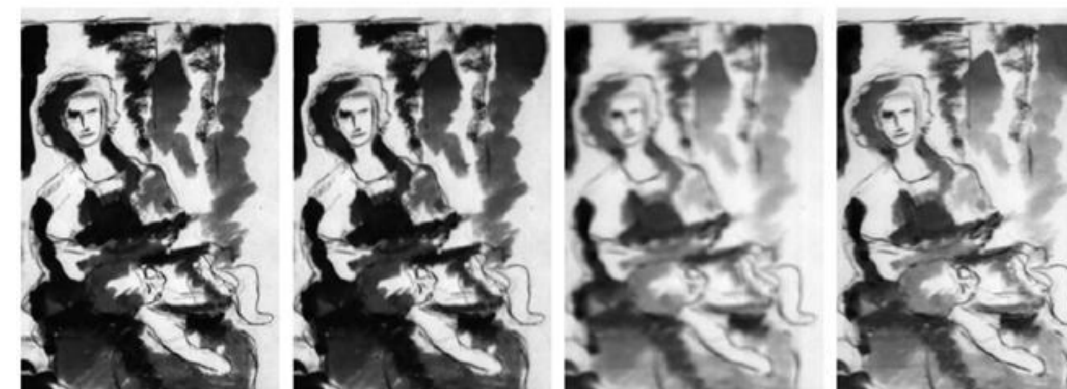
Figure 6: H 1 which is focused on the blue spectrum vs. H 2 which is focused on the red spectrum. (a) H 1 , channel 41 (457.82 nm), (b) H 2 , channel 41 (457.82 nm), (c) H 1 , channel 200 (854.97 nm), (d) H 2 , channel 200 (854.97 nm). Different focused channels. Solution? Spectral focus stacking.
