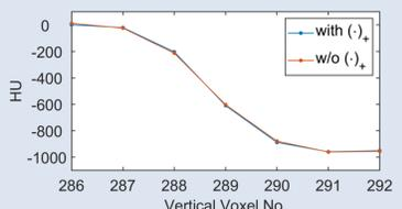
**Figure 4:** Profile plot for setting (c). Edge crossing from water to air, in HU.
