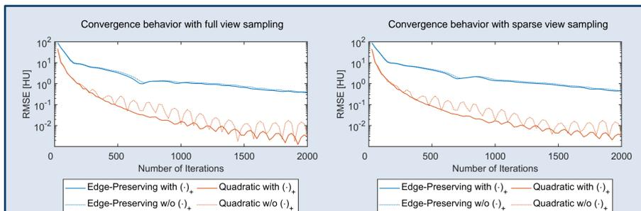
**Figure 5:** Convergence behavior for reconstruction of module A with full view sampling (left) and sparse view sampling (right). RMSE is calculated inside the phantom including its edges. Same curves are observed for module D.
