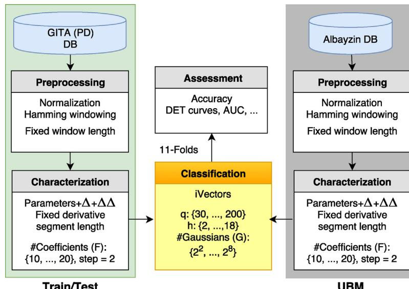
**Fig. 9.** i-Vectors training methodology outline. Features can be MFCC, Rasta-PLP and LPC with derivative coefficients  $\Delta + \Delta\Delta$ .
