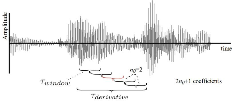
**Fig. 3.** Scheme illustrating  $\tau_{derivative}$  and its relationship with  $\tau_{window}$  and the number of coefficients used to calculate  $\Delta$  for  $n_0 = 2$ .
