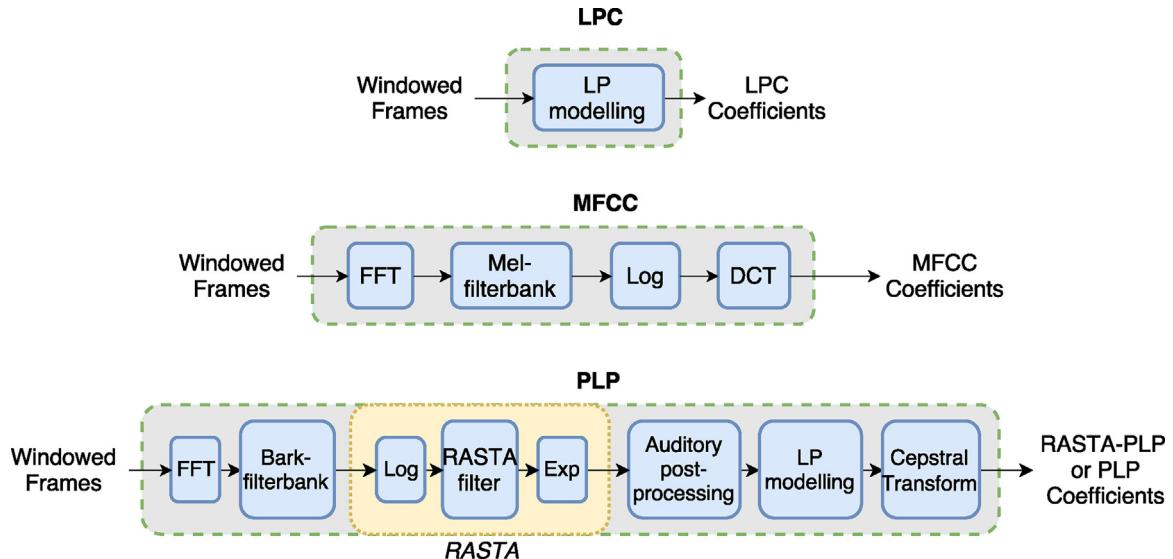
Fig. 2. LPC, MFCC and PLP calculation procedure scheme.
