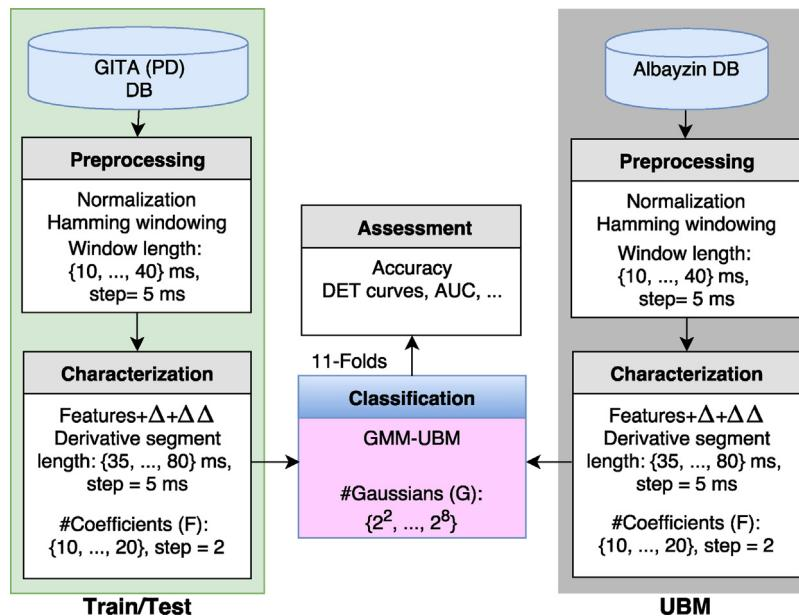
**Fig. 8.** GMM-UBM training methodology outline. Features can be MFCC, Rasta-PLP and LPC and derivative coefficients  $\Delta + \Delta\Delta$ .
