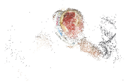
FIGURE 4: The obtained 3D point cloud from the SfM algorithm.
