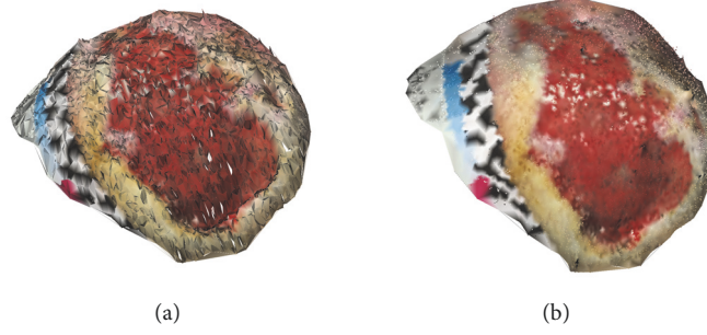
FIGURE 5: (a) The result of Delaunay triangulation algorithm which is a rough surface including some holes. (b) The smooth and integrated surface after filtering.
