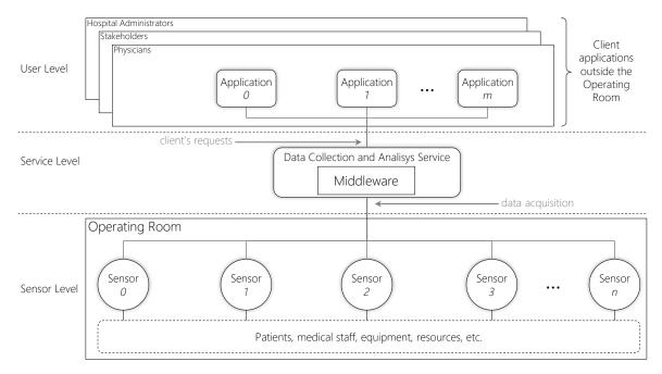
**Figure 1.** A monitored Operating Room model with a middleware acquiring and providing information in real time for user applications. The middleware is present in the service level, which can be deployed in a server or datacenter. As the number *m* user applications and *n* sensors increase, the middleware may decrease performance and consequently QoS.
