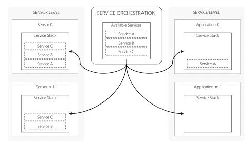
Figure 10. Example of the service orchestration process performed by the Orchestration Engine.
