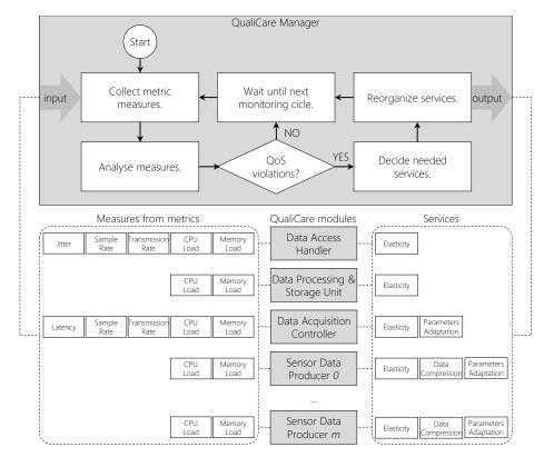
**Figure 8.** QualiCare Manager main monitoring cycle showing the service distribution and the metrics it evaluaves. The idea is to monitor module metrics and organize services according to the measures.
