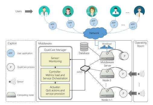
**Figure 5.** QualiCare closed-loop model with a Manager in charge of monitoring and adapting the middleware according to the workload. At the user perspective, *a* denotes the number of user applications. At the middleware perspective, *n* denotes the number of nodes running a QualiCare process that acquires data from sensors in the OR.
