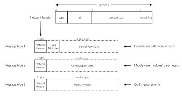
**Figure 4.** QualiCare message types and its contents. All messages use the same network header, which identifies the packets.
