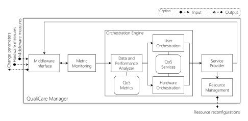
**Figure 7.** QualiCare Manager components, inputs, and outputs. The module receives measurements collected from the middleware and evaluates them based on metrics and services. The output are resource and parameters reconfigurations, if necessary, to guarantee QoS.
