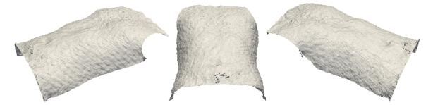
Figure 5.6: Qualitative results for RI data fusion and surface reconstruction for subject  $S_1$ . The subject was captured using two Kinect RI sensors. The proposed fusion and reconstruction framework enables a high coverage body surface model, however, the mesh reflects the noise characteristics of the RI device and exhibits artifacts due to sensor interference.
