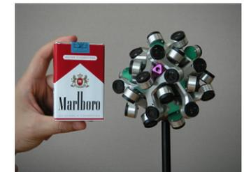
The Jupiter model is composed of 20 stereo units. It requires 10 PCs to process the stereo data.
