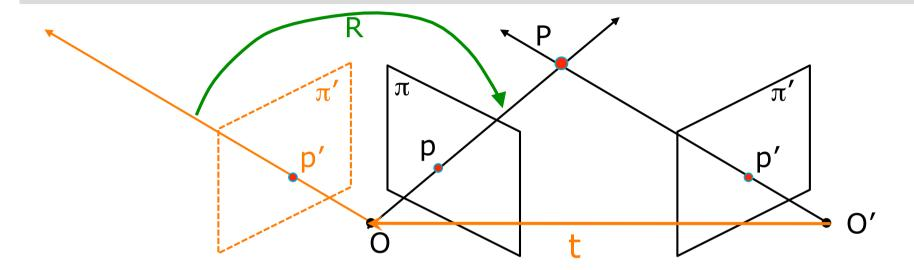
■ Still the two coordinate systems can differ by a rotation. Let *R* be the rotation matrix that aligns the corresponding axes of the two camera coordinates.
