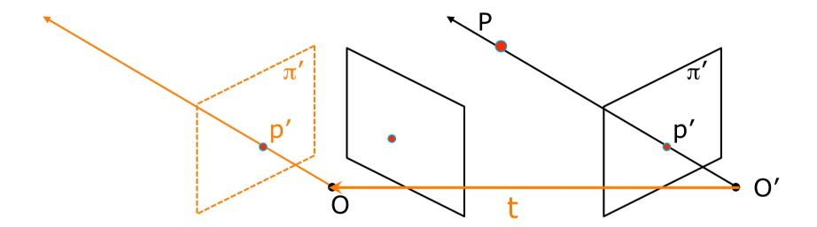
■ If we apply this translation *t* to every point *p'* of the camera with COP *O'* then we will move the coordinate system with COP *O'* so that both camera coordinates are pinned to the same origin *O*.
