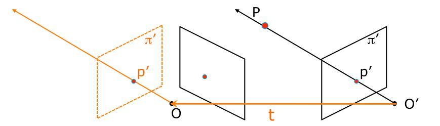
■ If we apply this translation *t* to every point *p'* of the camera with COP *O'* then we will move the coordinate system with COP *O'* so that both camera coordinates are pinned to the same origin *O*.
